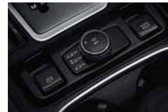
Electronic parking brake with auto-hold function
