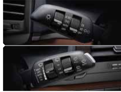
Headlamp control and automatic washer switches
