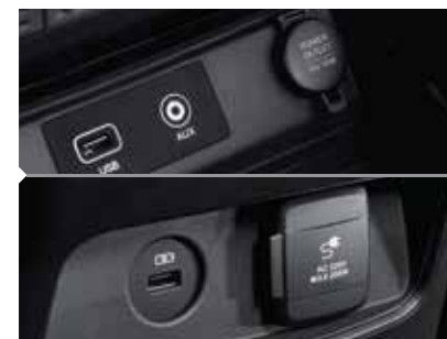
USB port and power outlet on centre console, USB port and 220V/115V inverter in 2 nd row
