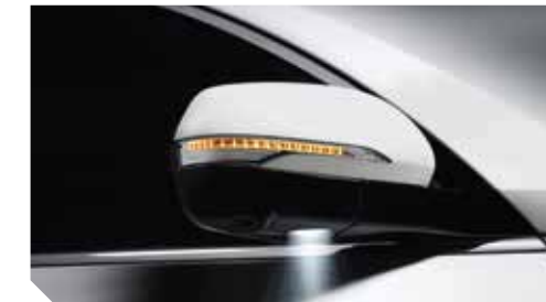
Side repeater and puddle lamp mounted on the back of the outside mirror
