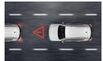
Forward Collision Warning (FCW) Alerts the driver when another vehicle or pedestrian appears in the path of the vehicle.
